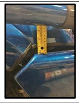
35. **CRITICAL:** Set distance from top face of the bull bar wing to bottom of rail to 85mm +/-2mm for correct set up.
