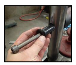
57. Install submerged bushing and M10 socket head cap screw.
