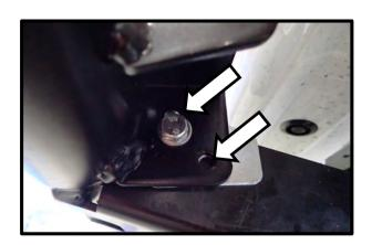
58. Tighten M8 bolt connecting the front rail to the step section ensuring the slot and holes in the spacers (if fitted) are aligned with the holes in the step sections and front rail.
