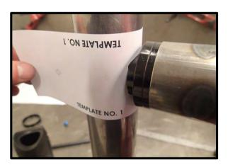
38. Swing the Side Rail inwards and install "TEMPLATE 1" between the end of the tube spigot and the Bull Bar outer frame
