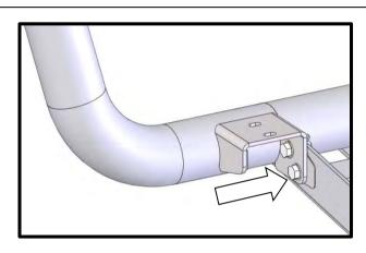
61. Pin the front side rail to the rear section using an M8x20 bolt, 2x M8 flat washers and an M8 nyloc nut.
