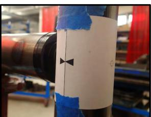
39. Carefully align and center "TEMPLATE 1" with the end of the tube spigot and wrap around the outer frame tube.
