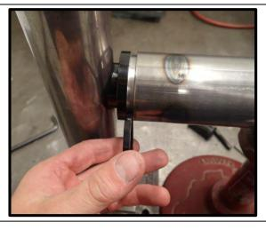
36. Assess the gap between the front end of the Side Rail and the tube spigot. Select the closest matching spacer/spacers to fill the gap. (Spacer options: None / 5mm / 10mm or 15mm (5mm + 10mm spacers).
