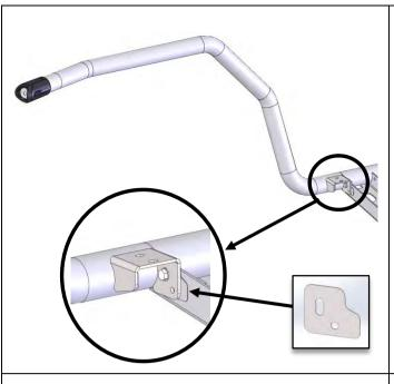
56. Install Side Rail (with clamp components fitted) onto Side Step spigot and attach using an M8x25 Bolt, 2x M8 flat washers and an M8 nyloc nut.
