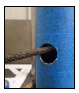
47. Using a small round or half-round file carefully remove any burrs from the edge of the Ø24mm hole.
