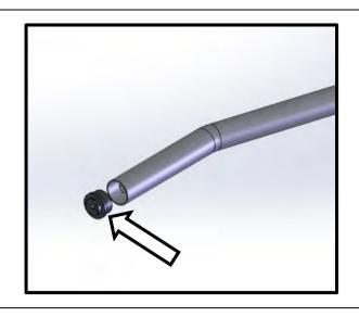
30. Install tube spigot into the front of the Side Rail – Install without spacers fitted.
