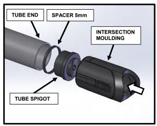
55. Install tube spigot, selected spacer/spacers and intersection moulding into place on the Side Rail.
