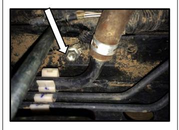
6. At the 765mm location on the driver side it is necessary to relocate the ground cable bolted to the top of the frame. Remove the hex screw and ground wire eyelet and reinstall on the opposite side of the frame using the same weld nut.
