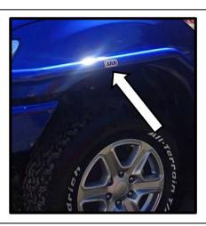
Apply the supplied ARB decals at the rear of the Side Step on both the RH and LH sides of the vehicle as indicated.
