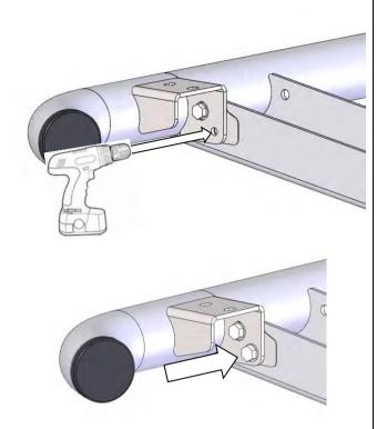
64 Using an electric drill with an Ø8mm drill bit, using the pre-cut hole in the Return Bracket as a guide, drill through the rear step section.
