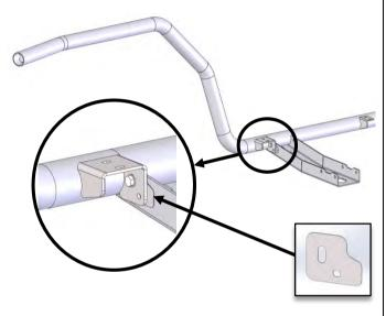
31. Place the Front Side Rail assembly onto the end of the Side Step Rear section as shown.
