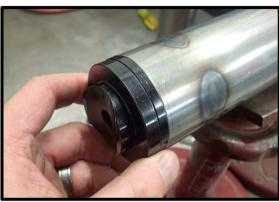
37. Swing the Side Rail outwards and away from the vehicle allowing installation of appropriate/selected spacer into gap between the front end of the Side Rail and the tube spigot. (5mm shown in this instance).
