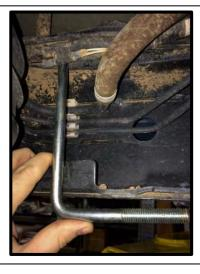
12. At the marked off locations on the driver side rail, insert the U-bolts upward between the wire harnesses and frame rail, as shown in the diagram, and then pivot the bolt so the threads point outwards.
