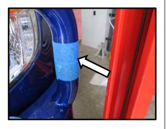
29. Use masking tape to wrap 1 x layer only of tape around the Bull Bar Outer Frame to protect it from damage. Ensure masking tape is applied flat and without creases.
